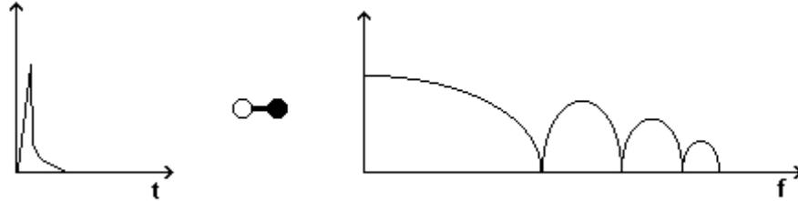
Figure 3.5: Hammer blow and its frequency spectrum
